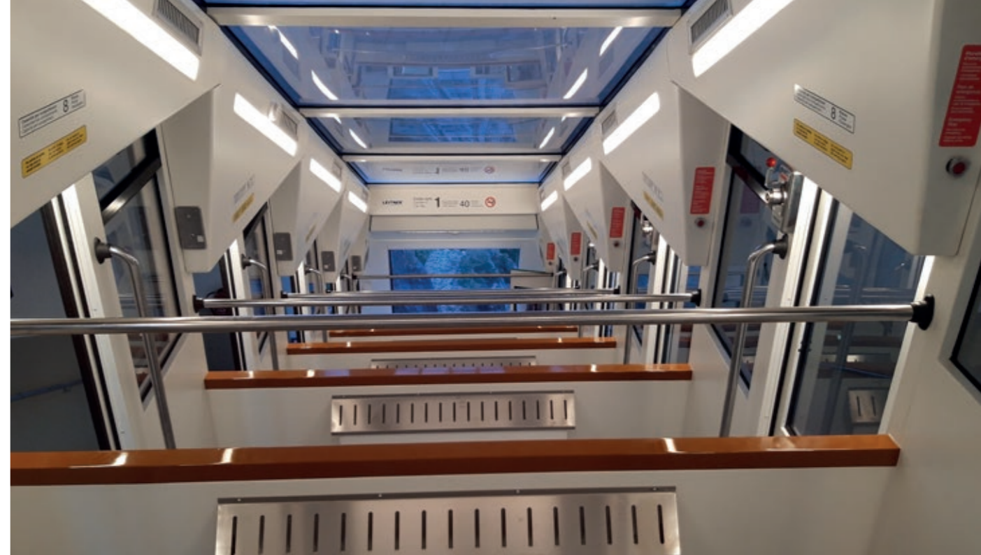
LEITNER SpA – Telefericos Y Nieve - Re-fitting of cable cars at Santa Cova – Montserrat – Spain. Cable car interiors - Compocel AL
